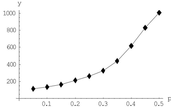
Fig. 2. The relationship between the number of the particles of the radius  $R$ , which have been trapped inside and the probability  $p$ , where  $p$  is the probability of assigning the wide channel of the filter
