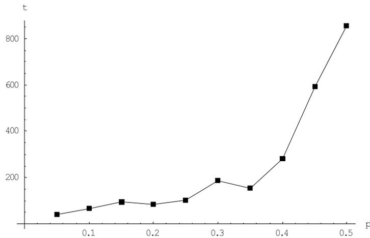
Fig. 4. The relationship between the time of the filter complete blocking and  $p$ , where  $p$  is the probability of assigning the wide channel of the filter
