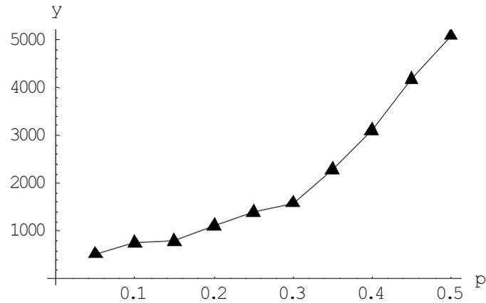
Fig. 3. The relationship between the number of all particles, which either have passed through the filter or have been trapped inside and  $p$ , where  $p$  is the probability of assigning the wide channel of the filter
