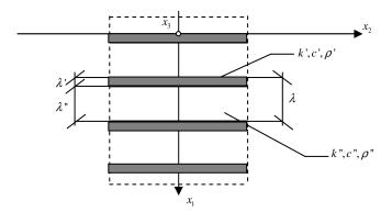
Fig. 1. A two-phased laminated medium
