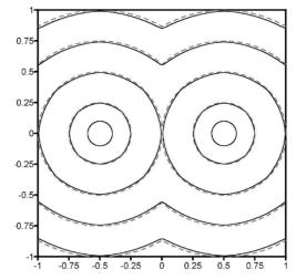
Fig. 4. The position of the interface at 0, 15, 40, 65, 90 s after the start
