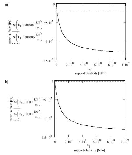
Fig. 4. The stress level in the upper face (S1 - solid line) and in the lower face (S2 - dashed line) as the function of the elasticity coefficient of the upper horizontal support  $k_1$ : a) elasticity coefficient of the lower horizontal support  $k_2 = 1\,000\,000\,\mathrm{kN/m}$ , b)  $k_2 = 10\,000\,\mathrm{kN/m}$
