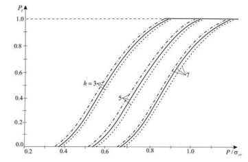
Fig. 7. Probability of failure of the composite for different values of the parameter *h* (solid for  $\eta = 0$ , dashed for  $\eta = 1$ , dotted dashed for  $\eta = -1$ )
