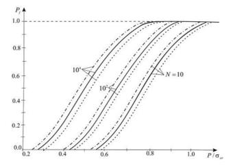
Fig. 6. Probability of failure for various types of stress state (solid for  $\eta = 0$ , dashed for  $\eta = 1$ , dotted dashed for  $\eta = -1$ )
