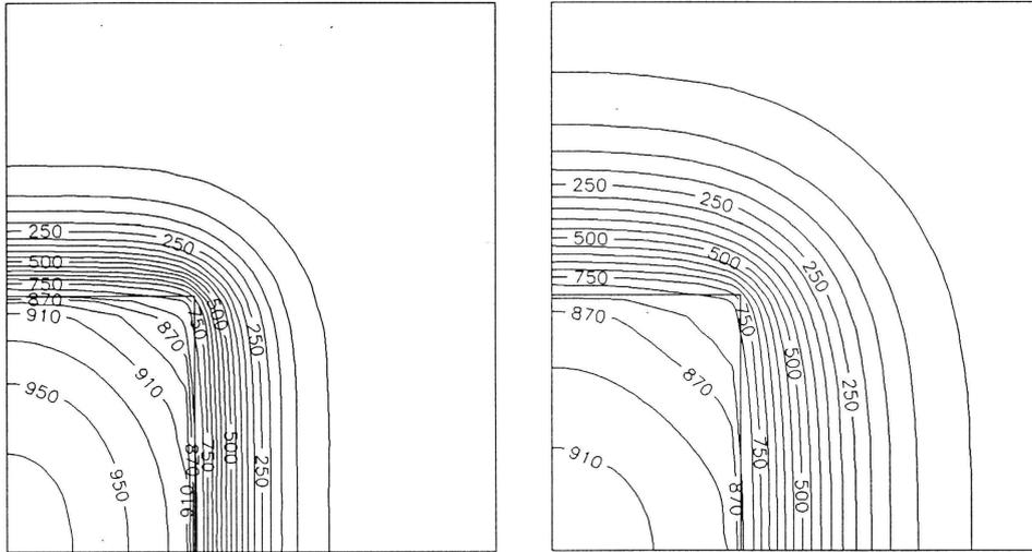
Fig. 1. Temperature field for 2 and 6 minutes
