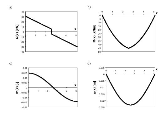
Fig. 2. The structural response of the beam: a) shear force, b) bending moment, c) slope, d) displacement function
