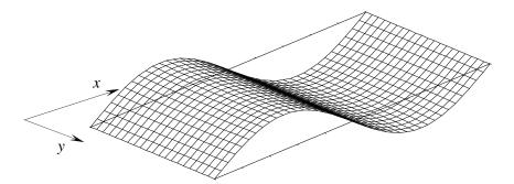
Fig. 12. The first buckling mode
