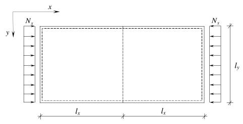
Fig. 15. A rectangular plate, simply-supported on all edges with one internal continuous support under constant normal loading
