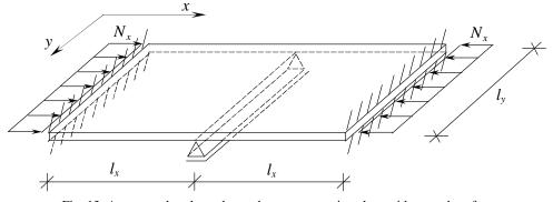
Fig. 13. A rectangular plate, clamped on two opposite edges with two edges free and one internal continuous support under constant normal loading
