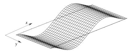
Fig. 14. The first buckling mode
