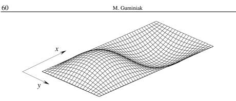
Fig. 16. The first buckling mode
