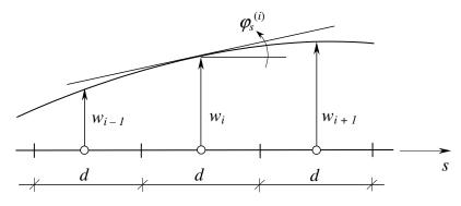
Fig. 6. Calculation of angle of rotation in tangent direction
