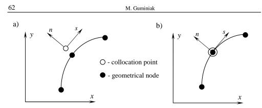
Fig. 2. Curved boundary element of constant type in non-singular and singular definition
