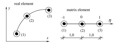
Fig. 3. Continuous, curved boundary element in singular formulation
