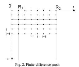
The differential form of equation (17) for the inner node *i* is as follows
