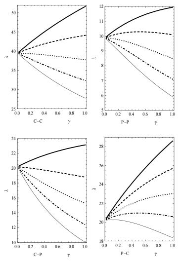
Fig. 1. Non-dimensional critical buckling loads with  $g(\xi) = (1 + \gamma \xi)^2$ ,  $h(\xi) = (1 + \gamma \xi)^{\alpha}$  as a function of  $\gamma$  for  $\alpha = 1$  (black bold line),  $\alpha = 1.5$  (dashed line),  $\alpha = 2$  (dotted line),  $\alpha = 3$  (black solid line) for different boundary conditions
