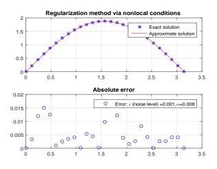
Fig. 4. v and  $v_{\alpha}^{\delta}$  with noisy data  $\varepsilon = 0.001$  for y = 0.7 and the absolute error
