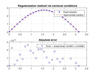
Fig. 5. v and  $v_{\alpha}^{\delta}$  with noisy data  $\varepsilon = 0.0001$  for y = 1 and the absolute error
