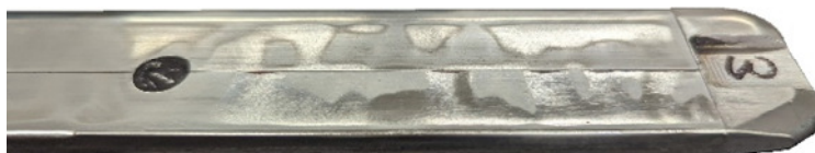
Fig. 4. Take-up bar rear ending, the original type a. The shading shows the problematic wavy surface after gluing the assembly
