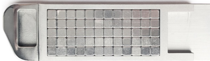
Fig. 3. The take-up bar (type c) stainless steel front ending with a block of magnets arranged in a Halbach array (state before assembling)
