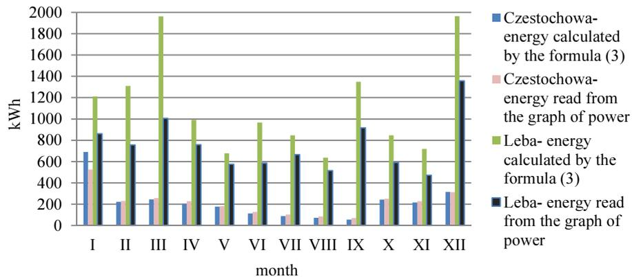
Fig. 6. The amount of energy produced by a single photovoltaic panel in Czestochowa and in Leba. The amount of energy calculated from the formula (3), compared with the amount of energy read from the graph of power [own calculations]
