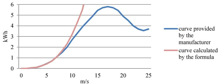
Fig. 5. Wind turbine power, read from the graph given by the manufacturer, compared with the power calculated by the formula [10-12]
