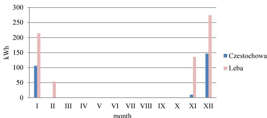
Fig. 3. Additional energy consumption to heat water in each month [own calculations]
