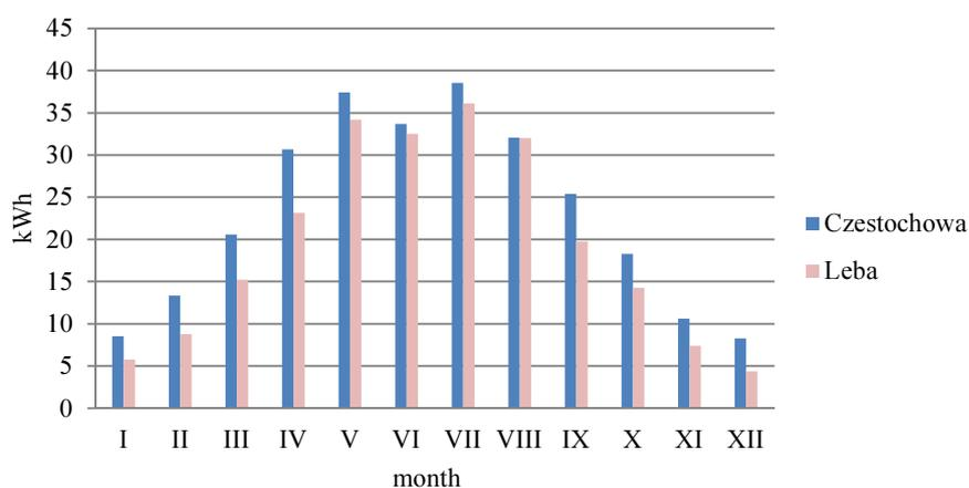
Fig. 4. Electrical energy generated by a single photovoltaic panel within a month in Czestochowa and Leba [own calculations]
