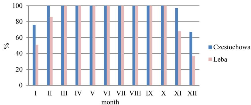
Fig. 2. Coverage of the energy requirements for heating hot water in each month. The energy produced by five solar collectors [own calculations]
